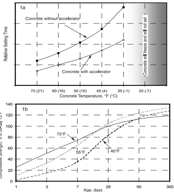
Figure 1 Effect of Temperature on Set Time (1a)
